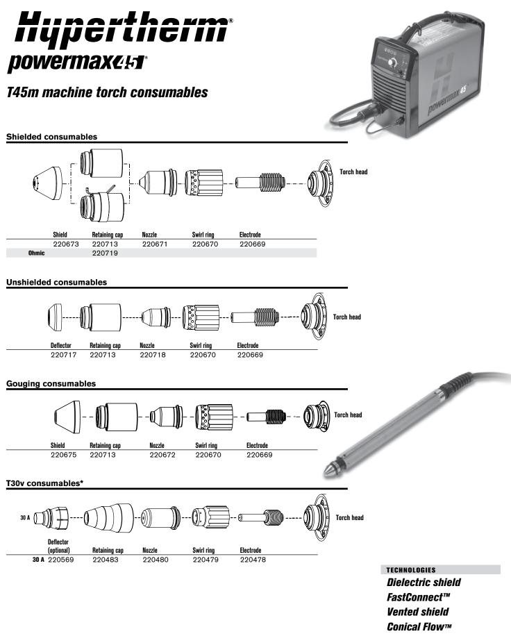
\* Use T30v 30 A consumables for 30 A fine-feature cutting on thin metals.
